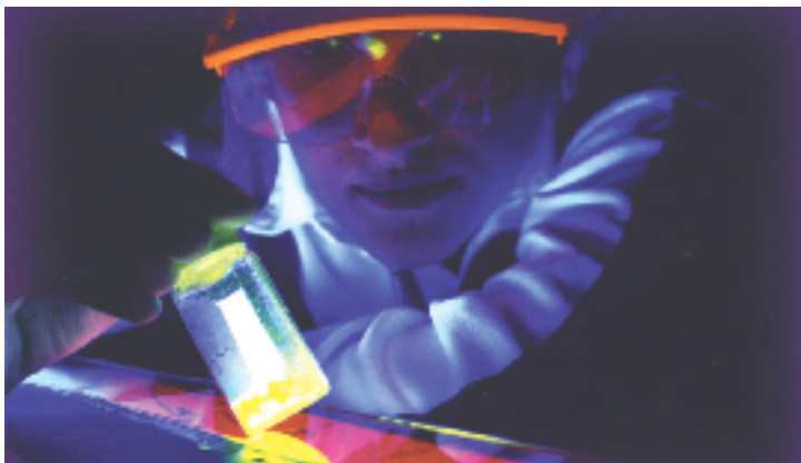
Amanda Aker, a chemical engineer with Nomadics, examines an amplifying fluorescent polymer under a black light. The polymer exhibits a dramatic reduction in fluorescence when exposed to traces of nitroaromatic explosives such as TNT. The polymer was engineered by research partners at the Massachusetts Institute of Technology (MIT), and is a key component of Nomadics' Landmine Detector and Advanced Sensors.
